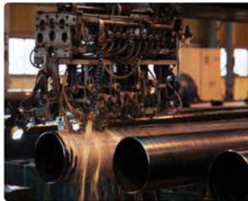
▲ Seam Ultrasonic Test (Off-line)
